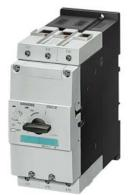
Circuit breaker size S3 for motor protection, Class 10 A-release 80...100 A Shortcircuit release 1235 A Screw terminal Standard switching capacity !!! Phased-out product !!! Successor is SIRIUS 3RV2 Preferred successor type is >>3RV2041-4MA10<<
